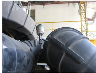
Image 5 - Potential Leak Sites on piping between air breather and turbo charger
