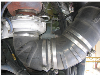
Image 5 - Potential Leak Sites on piping between air breather and turbo charger
