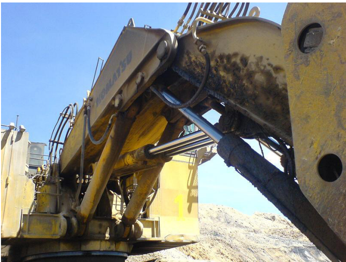
Image 13 - Hydraulic cylinders blocked in open position at end of stroke
