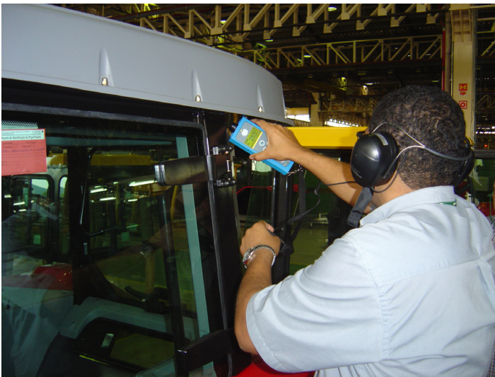
Image 18 - Ultrasound inspector checks for tightness of tractor cab at SIAC do Brasil with his SDT170 and SDT08 ultrasound transmitter
