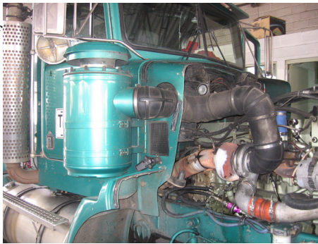
Image 4 - Typical Air Breather on Heavy Truck
