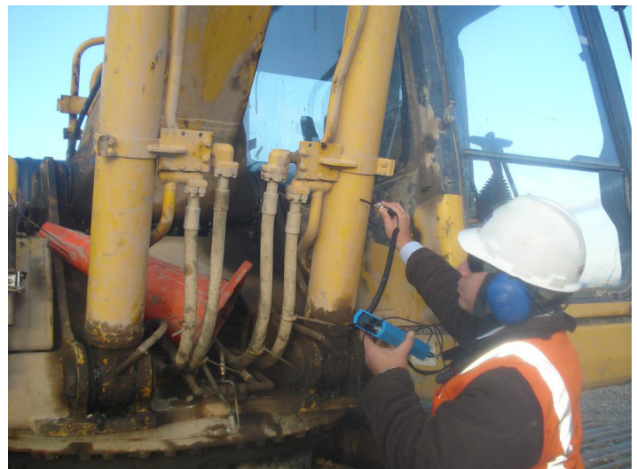
Image 14 - Place sensor on barrel of cylinder near piston
