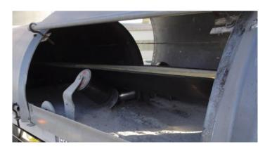
Since our vibration program is important in the plant, I wanted to integrate ultrasound into our existing predictive maintenance practices. That's when we came up with the idea of using it on our CB-1310 conveyor. At first, in 2016, we built a route only at the level of the return rollers. A reading on the roll frame gave us good signal quality for the application.
