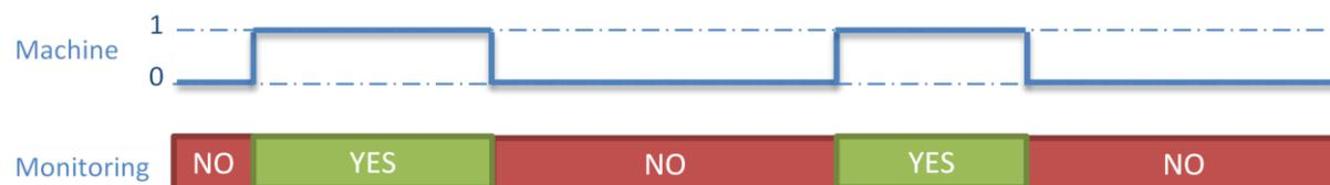
**Figure 71: Reliable monitoring periods are correlated to the machine running periods**
