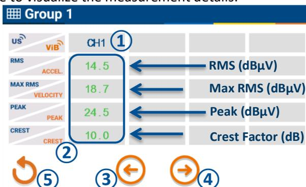
Figure 74: US readings, the channel number is in blue
