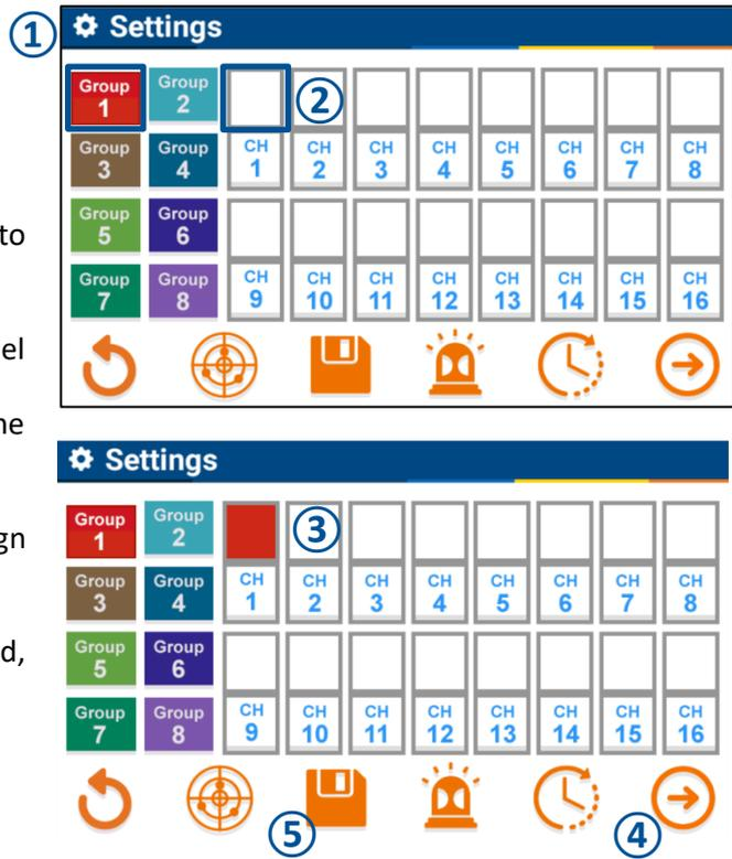
Figure 45: Channel assignment
