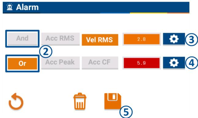
Figure 59: Adding condition indicator combination
