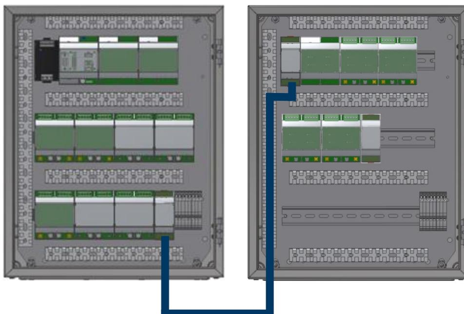
**Figure 21: The inter enclosure cable connects the expansion unit to the main unit**
