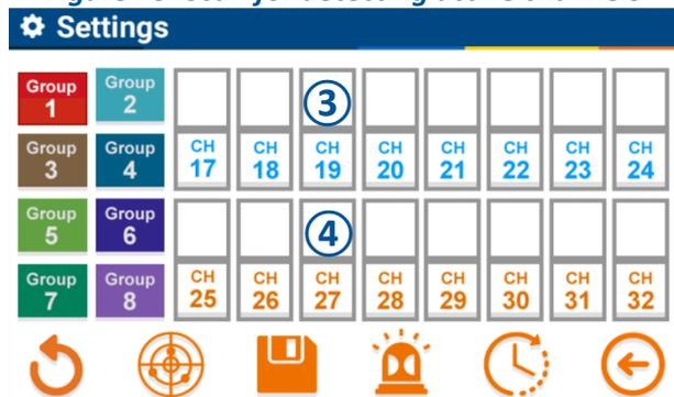
Figure 44: Active US channels are blue, VIB orange
