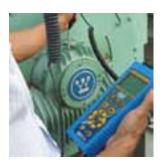
The most well-known trendable defect is condition-based bearing lubrication. It is a very simple and accepted science to trend using decibels. One basic thing to consider is identification of which bearings are greasable (yes, it is quite plausible to find a sealed bearing with a grease nipple). Other basic issues to consider include: Do you have the buy-in from your CMMS to migrate time-based lubrication, or will the
