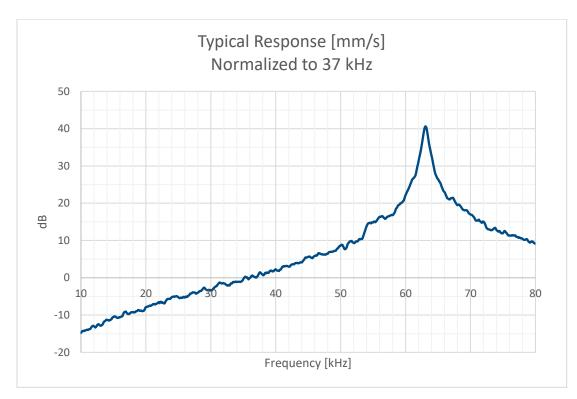
Typical response curve of airborne transducer:
