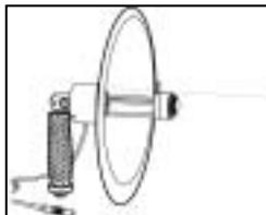
Figure 4 - Parabolic Sensor with Laser Sight
