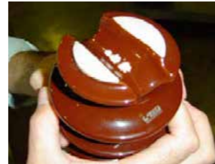
Figure 1: This insulator was damaged by tracking and eventually arcing. The problem was detected early with ultrasound inspection.
