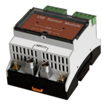
The VIB sensor module is the vibration conditioning and processing unit of the system. It collects analog vibration data (up to 2 sensors), computes all indicators and communicates this information to the main central unit.
